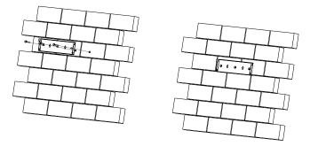
Figure 4.5 Mount the Rear Panel
