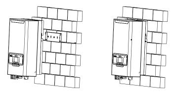
Figure 4.6 Mount the Inverter
