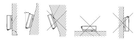
Figure 4.1 Mounting Method
