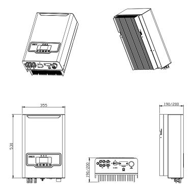
Figure 3.2 Dimensions of Sunttrio Plus 4K/5K/6K/8K/10K
